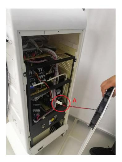
(3) Check the position of the Yag power supply: If it is on the right side, remove the right side of the case:
