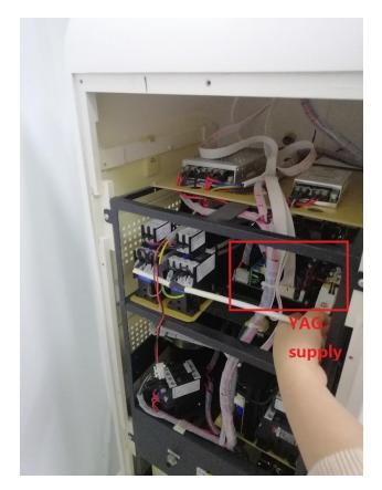
(4) Remove the right housing, you can see the Yag power position: As shown as the follow picture:
