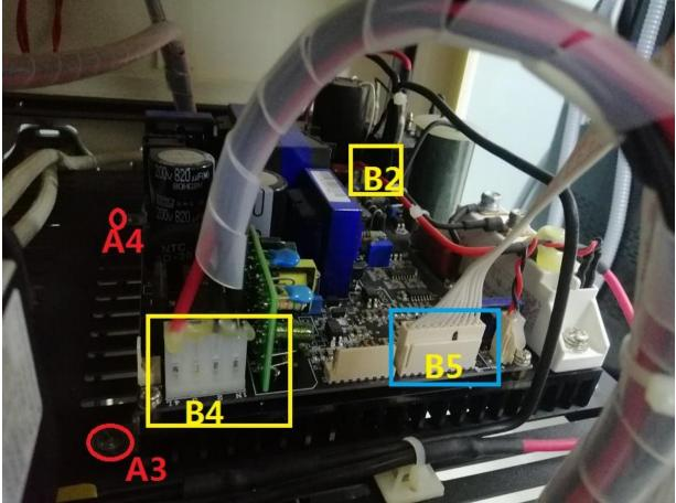
(6)Reinstall the new power supply,After installation, take a video and let me check whether the line is correct.
